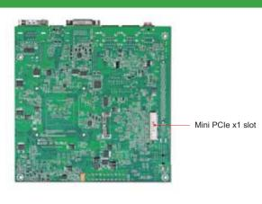
The WADE-8020 is built with the Intel® mobile QM57 chipset which works well with Intel® Core™ i5/i7 mobile processor technologies capable of supporting dual channel DDR3 memory. These features make the WADE-8020 the ideal solution for POS, Lottery, Medical, Gaming, High Resolution Digital Signage, Surveillance Security Monitoring, and Kiosk applications.
