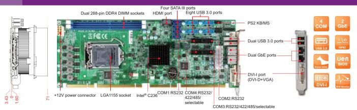
ROBO-8113VG2AR is based on Intel® C236 chipset and workstation processors. Built with flexible PCI express expansions, ROBO-8113VG2AR is suitable for Medical, Industrial automation, and Digital Signage application.
