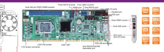
ROBO-8112VG2AR-Q87 is based on Intel<sup>®</sup> Q87 chipset and workstation processor sku like Core<sup>™</sup> i5/i7. Build with flexible PCI express expension, it's suitable for Medical, Industrial automation, and Digital Signage applications.
