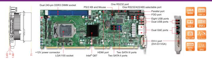
ROBO-8110VG2AR-Q67 is based on the Intel® Q67 chipset and desktop processor sku like Intel® Core™ i7 and i5. Built with flexible PCI express expansion, it's suitable for Medical, Industrial Automation, and Digital Signage applications.
