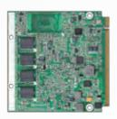
Qseven module based on Intel® Atom™ E640T/ E660T/ E680T platform with DDR2 SDRAM, four PCI Express lanes, 24bit LVDS, SDVO,CAN bus, NANDrive
