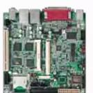
Mini-ITX Form Factor Carrier Board for Qseven Module with Dual Displays and Two GbE
