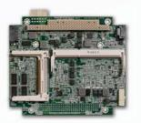
Portwell PEM-P393 is a PC/104-PLUS single board computer which uses Intel<sup>®</sup> Pineview N455 single core 1.66 GHz processor paired with the ICH8M I/O controller hub. It includes one SODIMM socket for DDR3 system memory and one Compact Flash socket.
