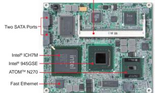
Portwell PEM-E200VLA is designed with Intel® N270 1.6 GHz processor with 945GSE and ICH7 chipset, with less then 10W overall TDP and dual 24bit LVDS support it is suitable for supermarket, health and industrial weighing scale applications which nowadays equipped with dual screen. For addition requirement the application will also require serial and USB ports to connect to thermal printer, barcode scanner to do self service while using weighing scale.
