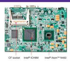
The PEB-2770/2780 takes advantage of the latest Intel® Atom™ technologies. It supports DDR2 SDRAM, dual gigabit ethernet and one expansion PCI Express x1 female header. Based on Intel® Atom™ solutions, the fanless PEB-2770/2780 executes high performance with low power dissipation. Therefore, it's applied to Panel PC, Kiosk, DS, Medical, Military and industrial automation.
