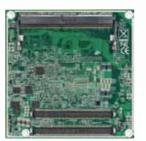
Intel® Skylake-U Core<sup>™</sup> i7/i5/i3 processor based on Type VI Compact-COM Express 2.0 module with DDR4 SDRAM on SO-DIMM slot, VGA, LVDS, Display-port, Gigabit Ethernet, PCIe, SATA, USB, OTG
