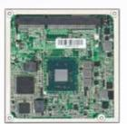
Intel® ATOM E3800 series based Type VI COM Express module with DDR3L SDRAM, VGA, eDP, HDMI, Gigabit Ethernet and 3Gbps SATA.
