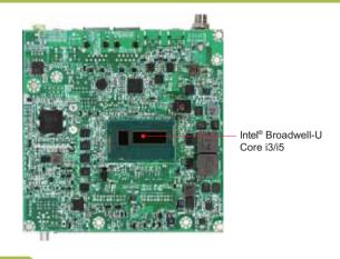
NANO-6050 build with Intel® 5th Gen Core™ i5/ i3 ULT processor and takes advantages of Intel® Core™ mobile processor technologies such as Hyper-Threading, high performance, and low power consumption. Portwell NANO-6050-based systems are ideal for passively cooled and hermetically sealed systems that can be used in various environments. NANO-6050 is an ideal platform with HD graphic output for POS, kiosk, digital signage and transportation applications.
